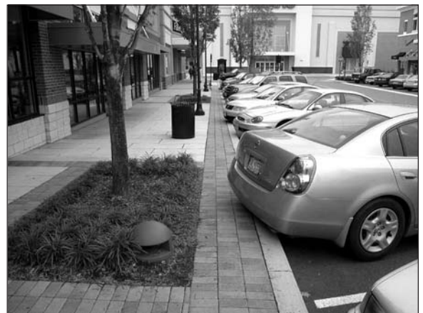
When on-street parking is used, planting areas should be separated from the curb to allow for vehicle overhanging and help preserve plantings from accidental damage.
