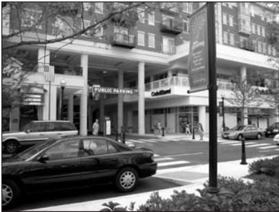
Retail and office uses should surround the ground level of parking structures to enhance the streetscape and create pedestrian-friendly environments.
